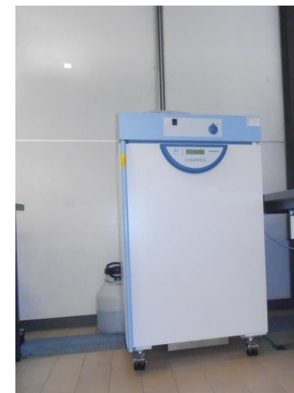
Climate chamber for simulating a temperature and humidity gradient
